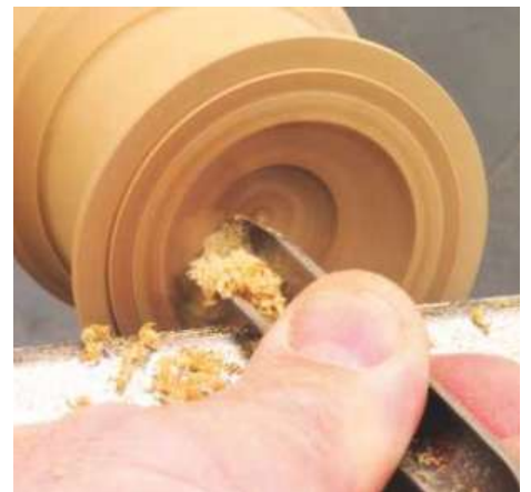
▲ Pic.9 With only half the outside shape done, hollow out the bowl section. A pull but with the spindle gouge is ideal, starting at the centre and drawing the tool towards you
